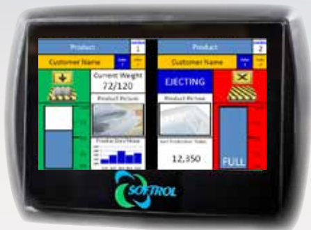
SmartStations provide the operator performance information
