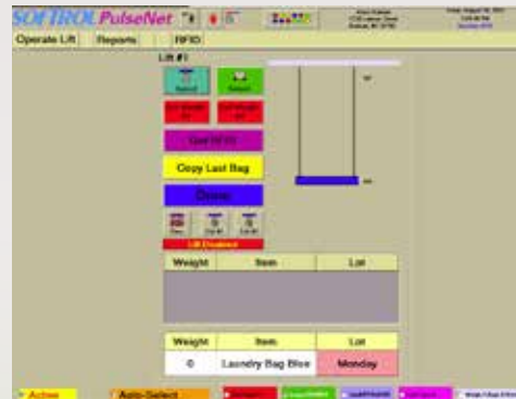
Lift lock-out for incorrect weights
