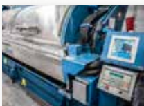
Water meters on individual washers monitor waster usage by machine
