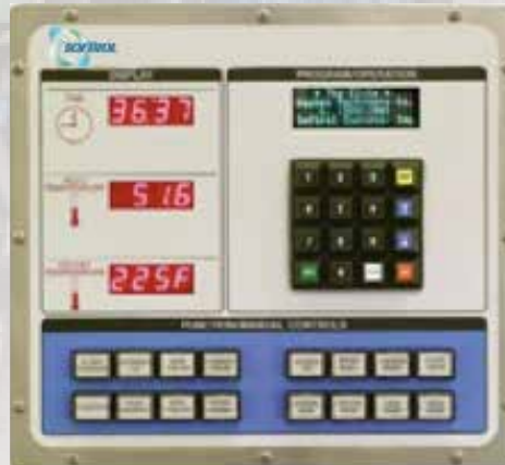
Automatically adjusts dryer time based on temperature change
