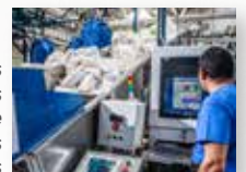
Control retrofits for tunnel washers help minimize the cost of continuous batch washers
