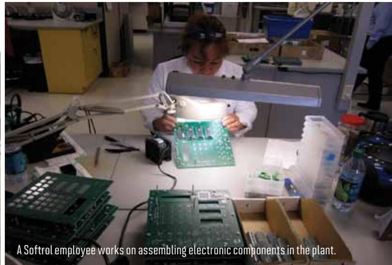
A Softrol employee works on assembling electronic components in the plant.
